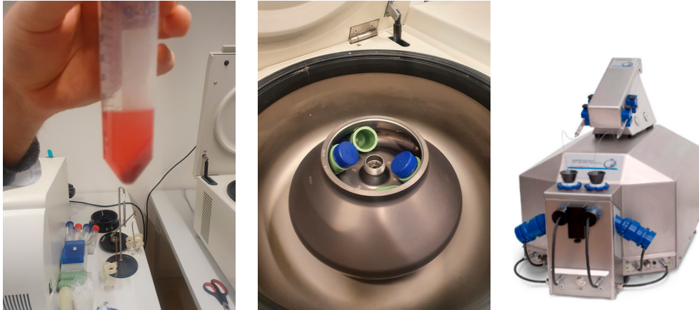
Fig. 2.4.1. Schematic representation of the sample preparation and measurement using high-resolution respirometry equipment for analysis of homogenized tissue (Oroboros instrument, Innsbruck, Austria)
