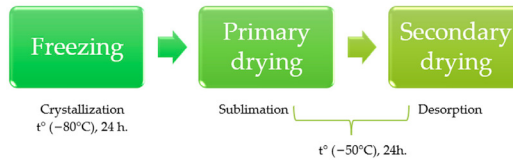
Figure 2. An overview of the three stages involved in the freeze-drying process.
