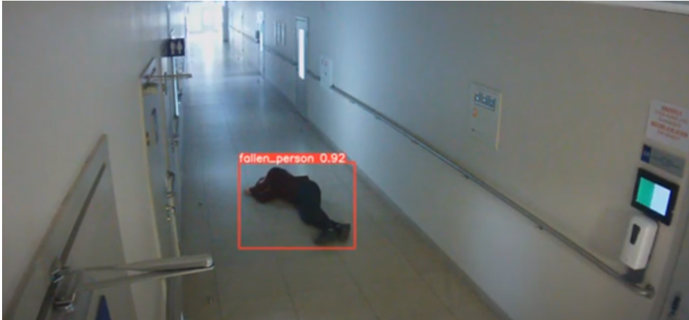
Fig. 3.3.1. Image from the performed experiment using artificial intelligence fall detection
