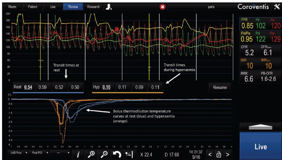
Fig. 3.6.1.3.2. Invasive physiological traces of pressure and temperature curves during bolus thermodilution displayed on a Coroflow console (Coroventis; Abbott)
