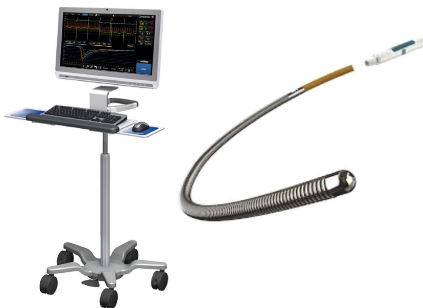
Fig. 3.6.1.2.1. CoroFlow coroventis system featuring the pressure wire X: a pressure/temperature sensor-tipped guidewire
