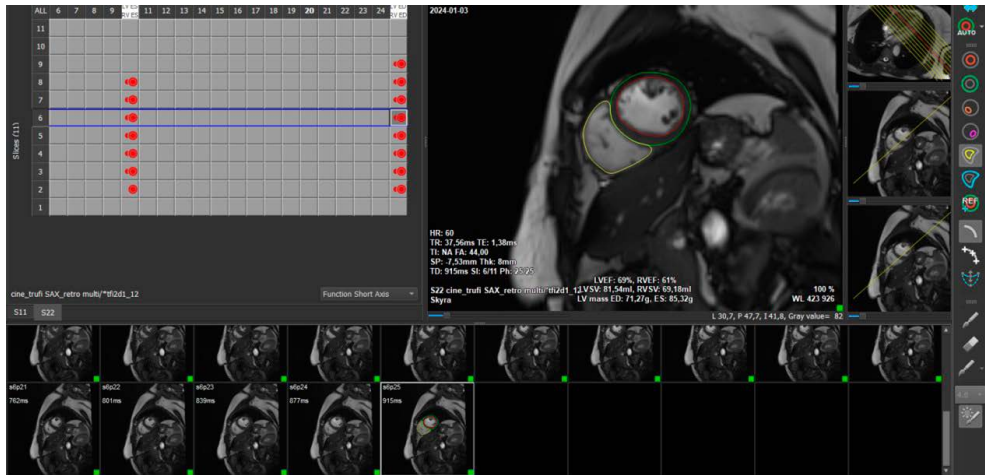
Fig. 2.6.1. Calculation of LV and RV volumes, LV mass and LV and RV EF.
